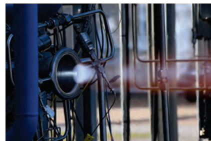
Hot fire testing of 3D-printed rocket nozzle at NASA.
