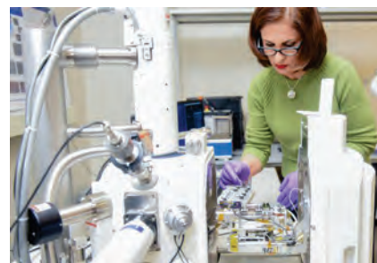
Afsaneh Rabiei and the device she developed to capture SEM images in real time at temperatures up to 1000°C.
