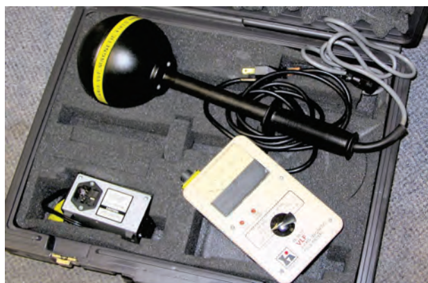
Fig. 2 — Holaday 3-axis VLF Magnetic Field Meter HI-3637.
