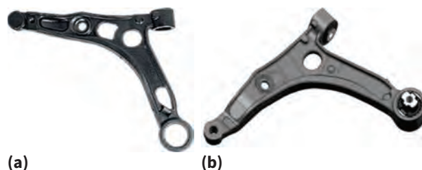
Fig. 3 — (a) Austempered ductile iron (ISO 17804/JS/900-S) suspension arm provides weight savings (5.9 kg machined weight versus 8 kg) and strength (600 MPa yield, 900 MPa tensile, 8% elong. versus 370 MPa, 590 tensile, and 10% elong.) over the (b) GH 60-38-10 pearlitic-ferritic cast iron version.
