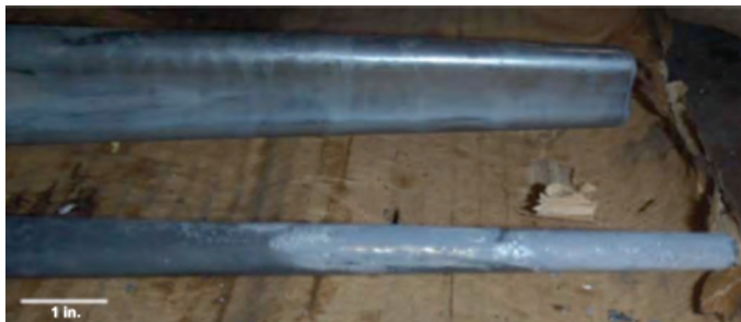
Fig. 5 — Steel slide inserts used in the production of a die cast driveshaft housing after 1256 shots [4] . The upper core with a 5- \mu m thick AlCrN coating shows no soldering, while the lower uncoated insert shows soldering.
