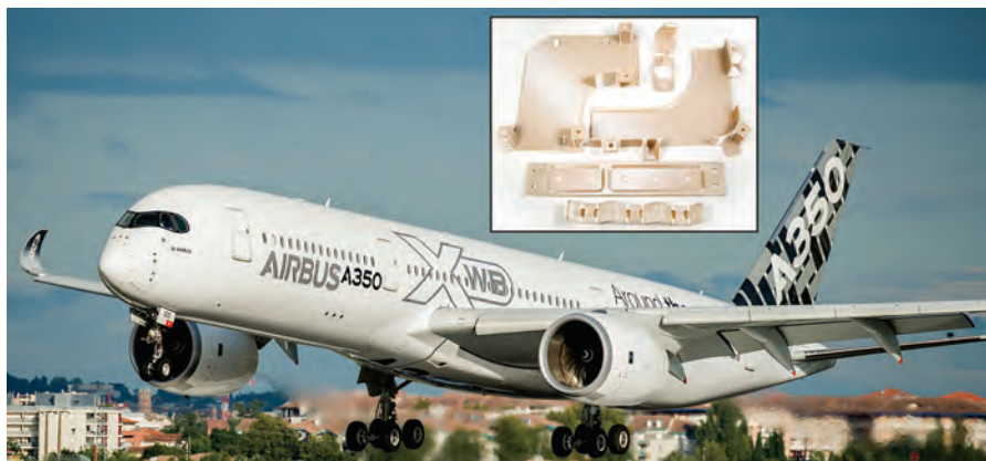
Airbus has qualified several 3D-printed polymer parts for nonstructural applications on its A350 XWB airframe. Courtesy of Airbus/Master Films/P. Pigeyre.
