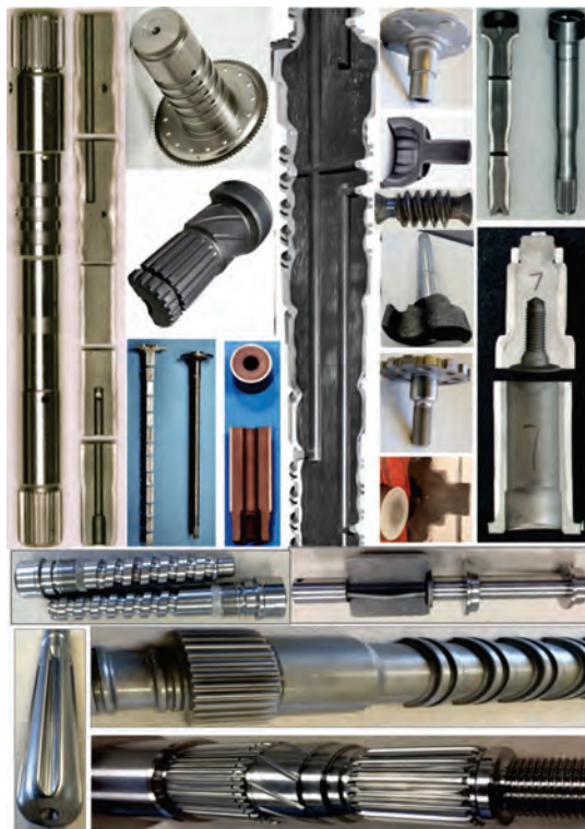
Fig. 2 — Examples of the variety of part geometries in modern shaft-like components.
