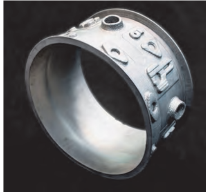
Fig. 6 — 24-in. diameter Inconel housing for turbine engine built using DM3D Technology's TransFormAM.
