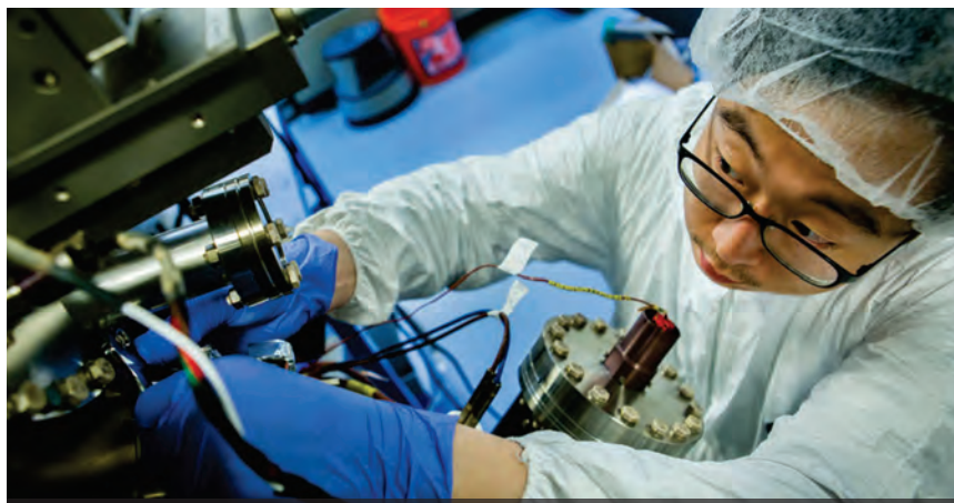
Graduate student Sunyeol Jun calibrates the molecular beam epitaxy apparatus used to characterize various semiconductors. Courtesy of Joseph Xu.
