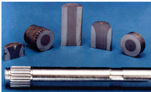
Fig. 1 — Representative shaft-like component induction hardened a decade ago.
