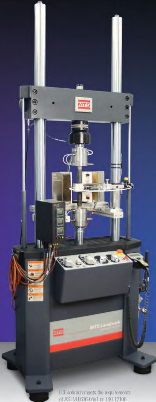
MTS Thermomechanical Fatigue (TMF) testing solutions supports temperatures up to 1200 °C
