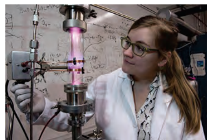
Samantha Ehrenberg uses a plasma reactor to create silicon nanoparticles for use in luminescent solar concentrators. Courtesy of Patrick O’Leary.
