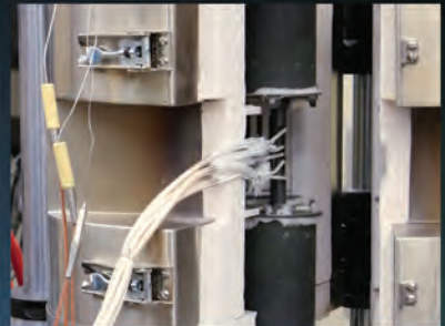
MTS high-temperature solution profiling a button head metallic specimen in 1200 °C
