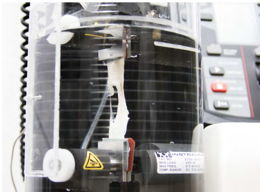
Tensile testing of biological tissues.
