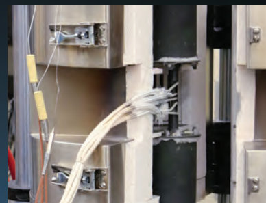
MTS high-temperature solution profiling a button head metallic specimen in 1200 °C
