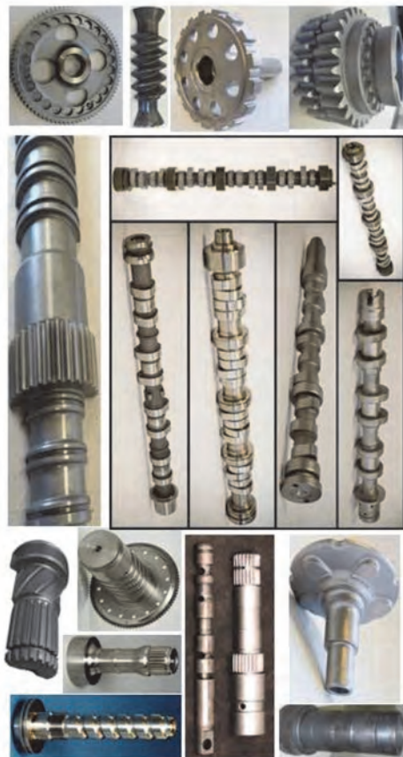
Fig. 1 — Variety of complex geometry components that are routinely induction hardened.
