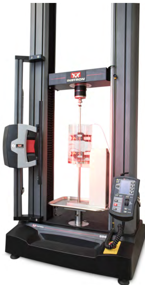
Tensile testing of hydrogels using a video extensometer.
