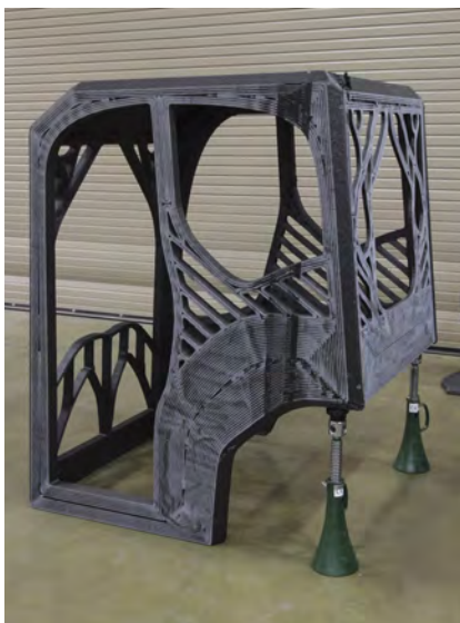
3D-printed excavator made of carbon fiber-reinforced ABS plastic. Courtesy of ORNL.
