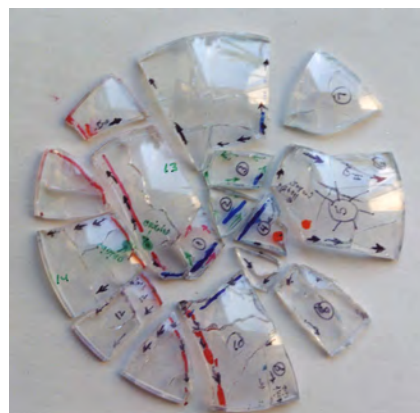
Fracture of a sapphire dome. Courtesy of NIST.
