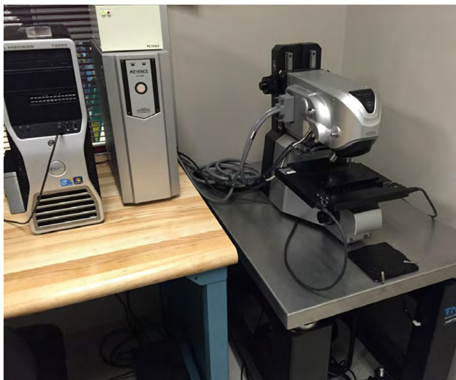
Fig. 1 — Keyence VK-X laser microscope.
