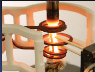
MTS Thermomechanical Fatigue (TMF) testing solutions supports temperatures up to 1200 °C
