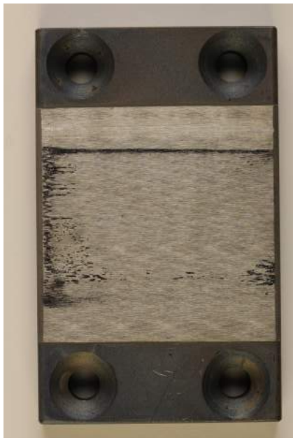
High velocity oxygen fuel coated sample for strip draw test used to evaluate tribological performance.
