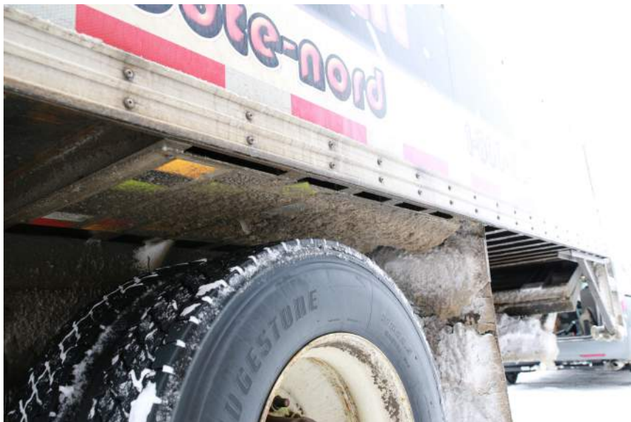
Painted aluminum samples exposed to in-service conditions for determination of chipping and blistering resistance.
