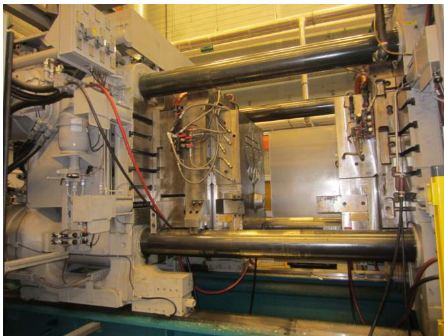
Fig. 1 — Clamp area of 1200-ton, high-pressure die casting machine used for industrial-size trials at CanmetMaterials facility.
