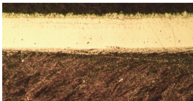
Fig. 6 — Boride layer on wrought Inconel 718 test bar. Boride layer depth range: 0.0012-0.0013 in. Boride layer hardness (three locations): 3014, 2778, and 2892 HV (50 g load). Etchant: Marble's reagent. Original magnification 200x.
