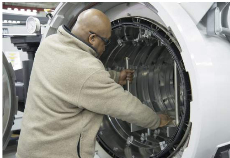
A key step for performing a successful Temperature Uniformity Survey is ensuring the survey fixture is carefully placed within the hot zone. Courtesy of Ipsen.
