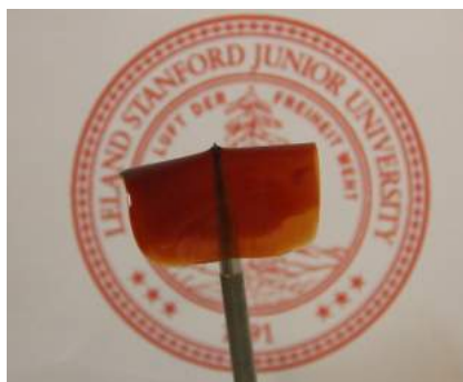
Jolting a new polymer material with an electrical field causes it to twitch in a muscle-like fashion. It can also stretch to 100 times its original length and repair itself if punctured.
