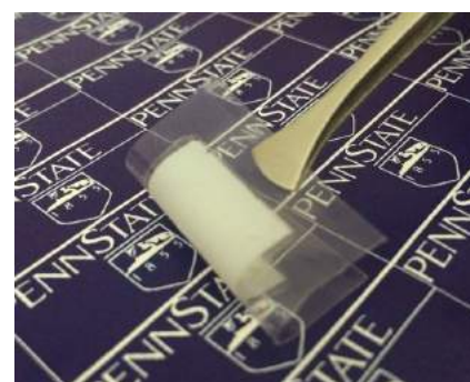
Flexible electrocaloric fabric of nanowire array can provide personal cooling. Courtesy of Qing Wang/Penn State.
