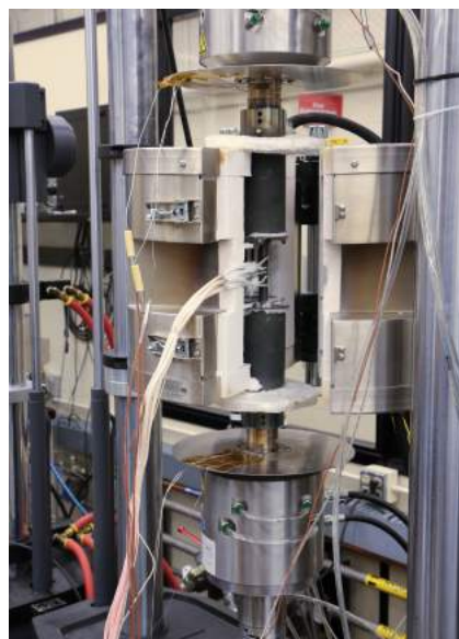
Temperature profiling of a button-head metallic specimen in 1200°C grips.
