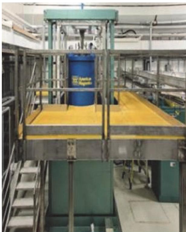
Fig. 3 —ORNL industrial prototype magnetic processing equipment includes 8-in. diam. vertical warm-bore superconducting magnet system and Ajax Tocco Magnethermic 200-kW dual-frequency induction heating system with 75-gpm polymer-water quench.
