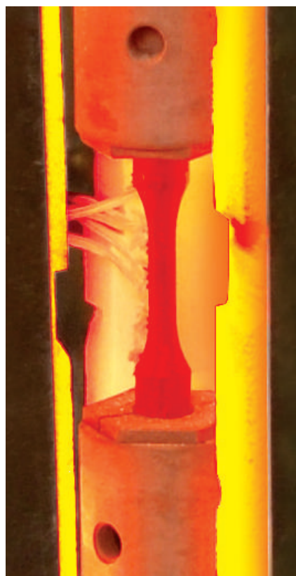
Thermocouples bonded to the specimen are used to measure thermal gradients.
