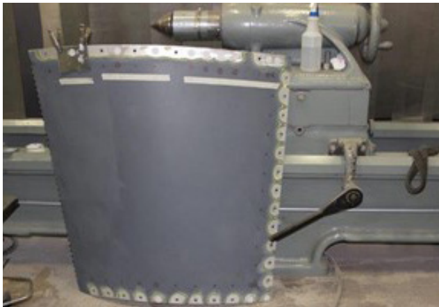
Fig. 5 — Aluminum repair on lightweight aircraft panel. Courtesy of ASB Industries.
