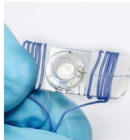
Prototype of an electrically switchable contact lens made of liquid crystals.
