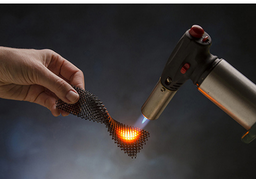
A new ceramic resin can be 3D printed into parts of any size. Courtesy of HRL Labs/Dan Little Photography.
