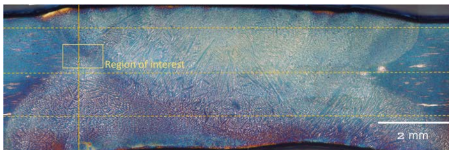
Fig. 2 — Polarized LOM mosaic image of a weld with investigated region marked by a square. Dotted lines represent points where hardness measurements were performed. A marked segregation appears at the edge of the fusion zone boundary, indicated by color change.
