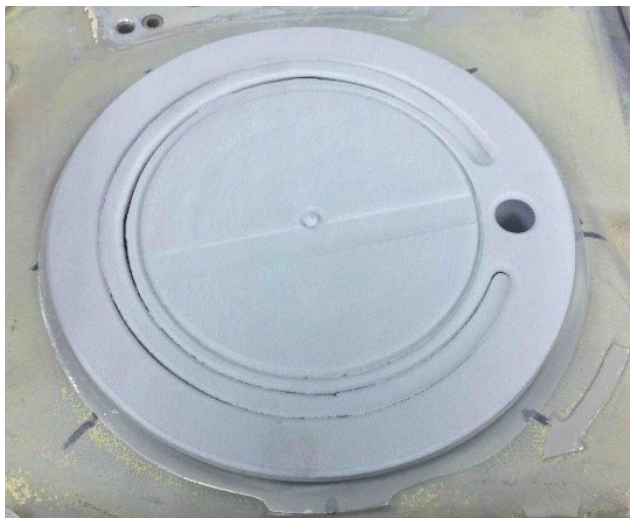
Fig. 2 — Hydraulic pump pad in the as-sprayed condition shows the AA4047 coating. Courtesy of Applied Research Laboratory, Penn State.
