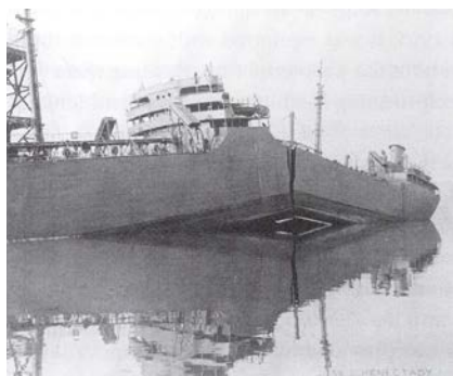
SS Schenectady, a welded tanker ship that broke in half while docked in 1943.
