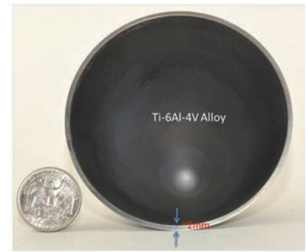
Fig. 8 — Fabrication of net-shape hollow cone made of Ti alloy produced by FAST ( 1200^\circ\text{C} , 25 MPa, 5 min hold time).
