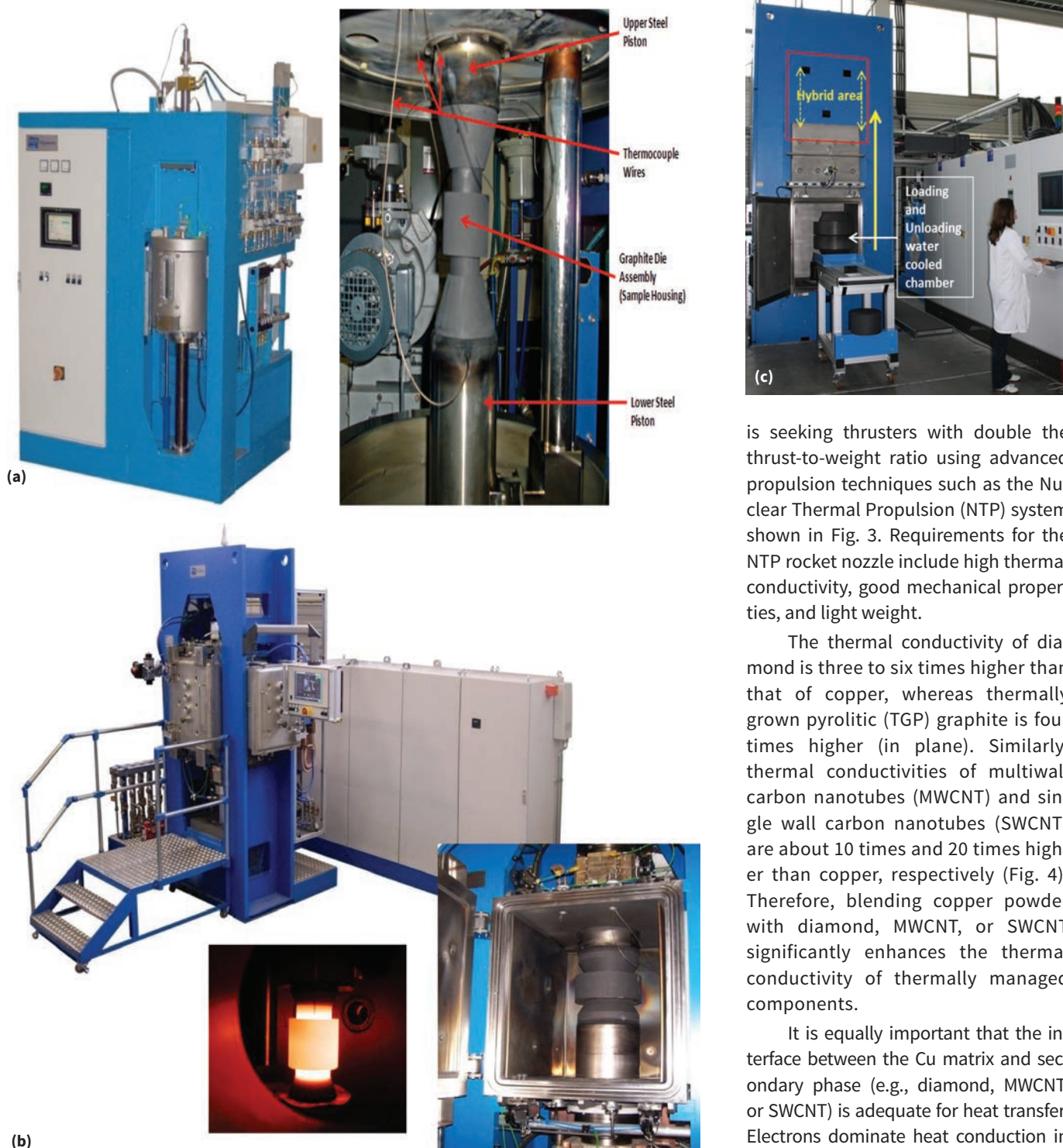
Fig. 2 — Field-assisted sintering units: (a) 25 ton, (b) 250 ton, (c) hybrid 320 ton.
