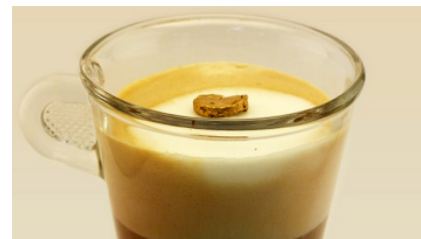
Twenty carats of gold foam is lighter than milk foam. Courtesy of Gustav Nyström and Raffaele Mezzenga/ETH Zurich.
