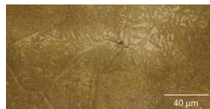
Fig. 8 — LOM mosaic image of Detail (b) in Fig. 6 shows coarse retained austenite regions. Etched with Vilella's reagent.
