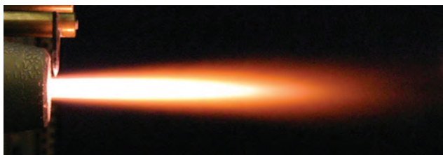
Color of the HVOF flame during spraying of suspensions starting from an \text{Al}_2\text{O}_3 powder with alkali impurities.
