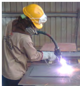
Fig. 3 — Thermal spray aluminum coating application in progress on test panel.
