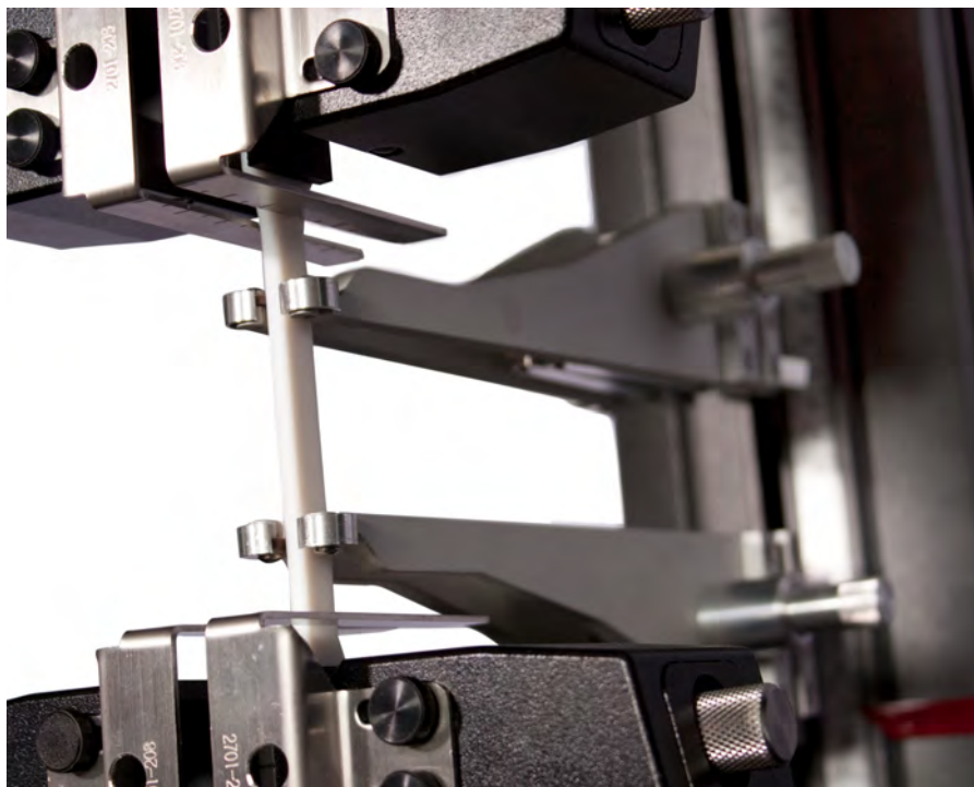
Fig. 6 — Automatic extensometers reduce setup time as desired gauge length is automatically set.
