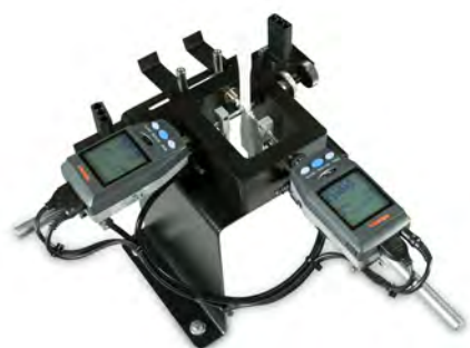
Fig. 5 — An automated measurement device measures width and thickness at the same time.
