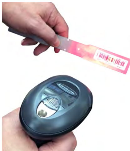
Fig. 3 — Barcode labeling and a barcode reader allow necessary batch and sample information to be loaded into a testing system or LIMS by scanning a barcode.
