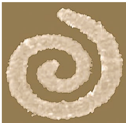
Scanning electron microscope image of a single gold nanospiral. Courtesy of Haglund Laboratory, Vanderbilt University.
