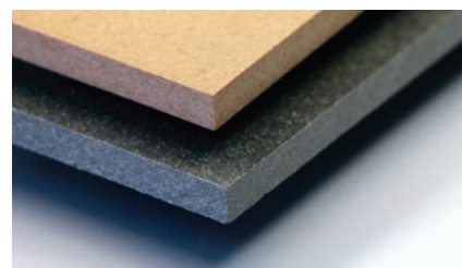
WPC board without (above) and with (below) flame-proofing. Courtesy of Fraunhofer WKI.
