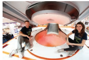
This 50-ton induction furnace from ABP Induction shipped to Saudi Arabia immediately following ThermProcess.
