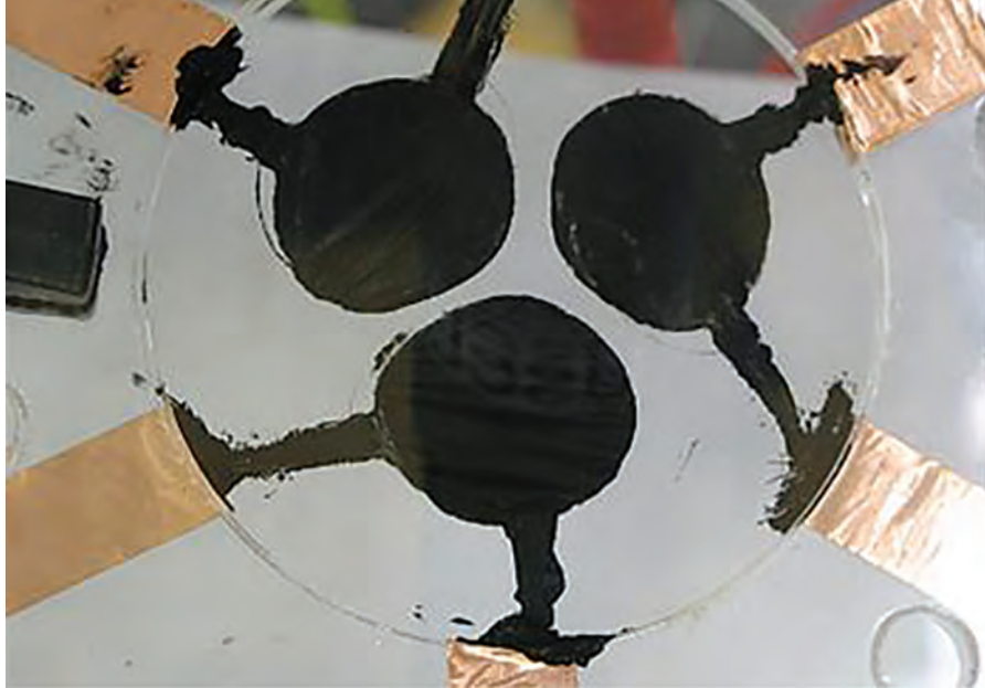
Three prototype artificial cephalopod chromatophores shown in unactuated states. Chromatophores are made of dielectric elastomer using tape coated with black carbon grease electrodes. Courtesy of University of Bristol.
