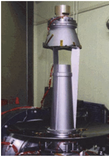
Fig. 5 — Prototype SIRTf telescope undergoing random vibration testing [5] .
