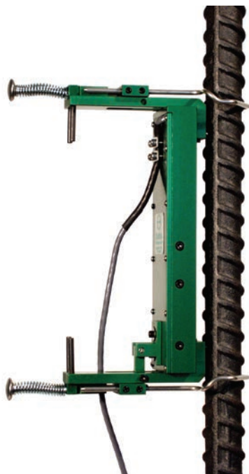
Manual, clip-on style rebar extensometer.
