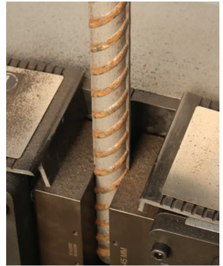
Abundant scale accumulation on lower grip after one test.
