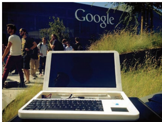
The Pi-Top, a laptop you 3D print yourself, has all the functions of a normal laptop.
