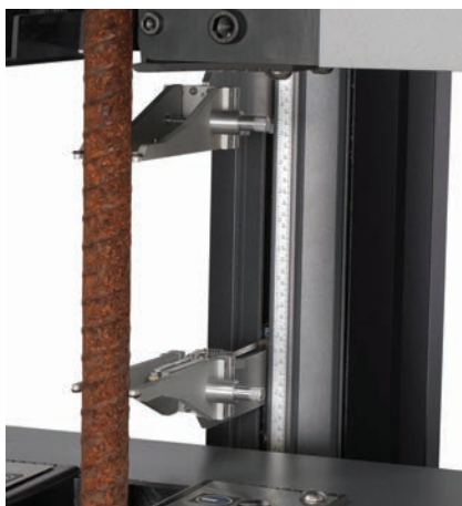
AutoX750 testing #11 (36 mm) rebar on an Instron 1500 KPX.
