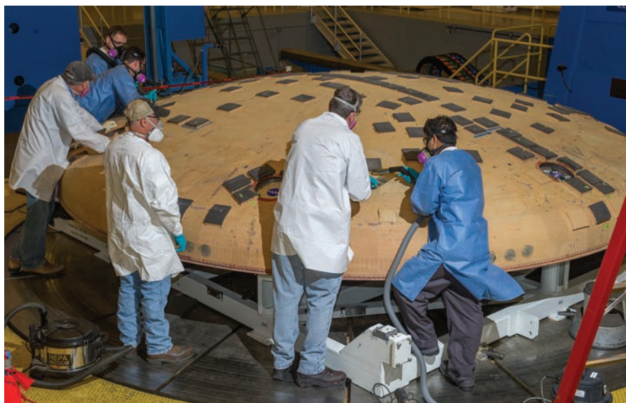
Engineers from NASA's Ames Research Center in Moffett Field, Calif., and NASA's Marshall Space Flight Center in Huntsville, Ala., remove segments of a heat-resistant material called Avcoat from the surface of the Orion heat shield. Courtesy of NASA.
