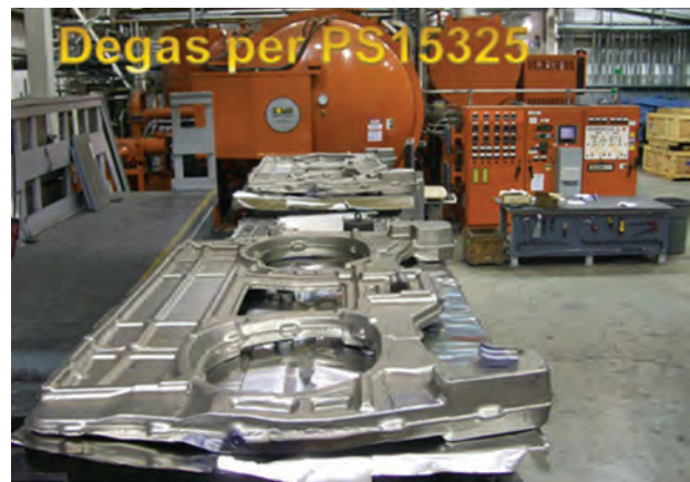
Fig. 12 — Titanium bulkhead forgings successfully processed in a graphite insulated vacuum furnace to meet final stringent surface contamination requirements.
