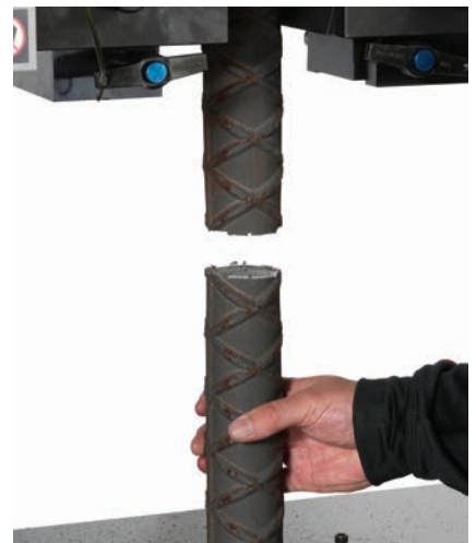
Number 18 (57 mm) bar separation (recoil) after failure.
