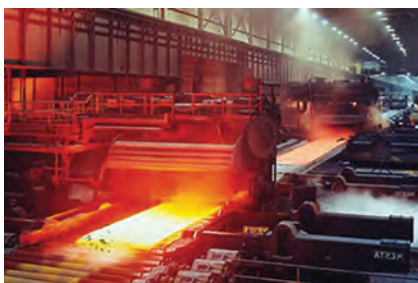
Hot rolling of sheets. Courtesy of Bethlehem/ISG and library.fordham.edu.
