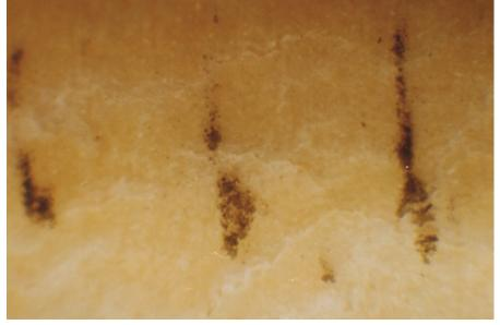
**Fig. 1** — Surface of a freshly baked bread roll shows black deposits at regular intervals. FTIR spectroscopic analysis determined that burnt deposits are associated with corn meal used as a release agent during the baking process.
