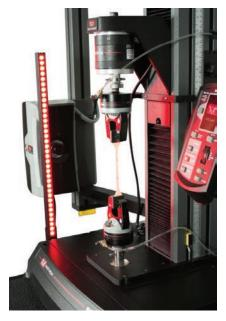
**Fig. 1** — Polarized LED lighting on the Instron AVE2 increases extensometer accuracy by removing ambient light effects.
