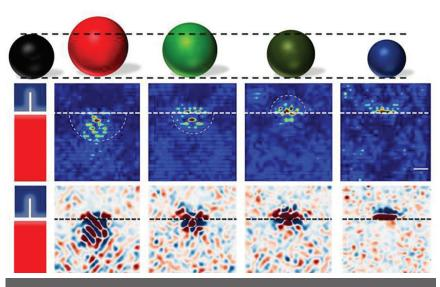
Simulations show the effects of dislocations in cerium dioxide on the redistribution of differently sized dopant atoms, replacing a cerium atom in the crystal lattice. Results reveal different amounts of segregation around the dislocation caused by the differently sized elements. The sizes of the other atoms are compared to a cesium atom (left, in black). The white dashed line shows the plane of the dislocation caused by strain. Courtesy of the researchers.
