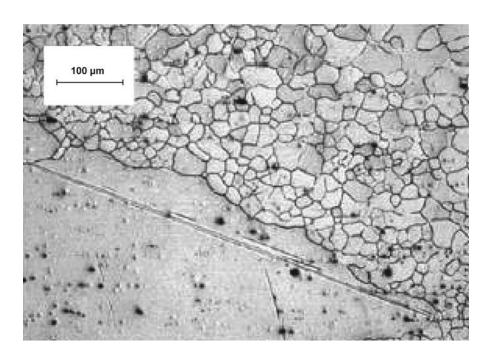
**Fig. 3** — The microstructure of the outer surface of an extruded AZ31 magnesium alloy showing the occurrence of abnormal grain growth when annealed to 450°C for three hours<sup>[30]</sup>.
