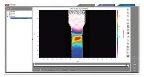
Fig. 4 — Digital image correlation analysis shows localized strain on a plastic tensile specimen.
