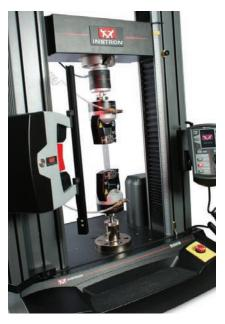
**Fig. 2** — Film testing conducted on the Instron AVE2.
