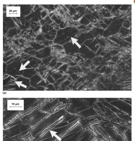
**Fig. 2** — Microstructures of AZ31 magnesium alloy rolled at 100°C and then annealed at 280°C for 10 s demonstrating (a) the presence of contraction twins and (b) nucleation at contraction twins<sup>[9]</sup>.
