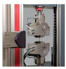
Hydraulic grips are able to clamp very small test specimens.
