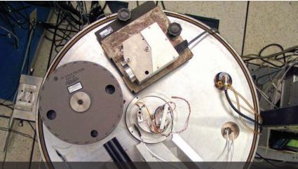
A laser from the NIST-designed autocollimator (square device at top) is beamed at the mirrored polygon in the gray circle at left, and its reflection allows the angle of the polygon's faces to be precisely determined while the polygon rotates. The black device at the bottom takes measurements that minimize wobbling by the polygon while spinning. Courtesy of Hudson/NIST.
