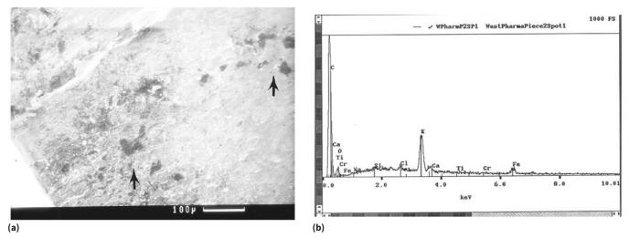
Fig. 4 – (a) SEM image at failure initiation zone with a ratchet showing clusters of inclusions and precipitates (arrows), mag: 160×, and (b) energy dispersive spectroscopy (EDS) spectrum of an inclusion indicates peaks for C, K, Ca, Cl, and Cr. This particle has probably come from the ironmaking operation in the blast furnace where sources for K are iron ore and coke ash while Ca is from the basic flux, such as lime (CaO), used for desulfurization of iron ore.
