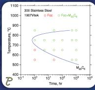
TC-PRISMA calculated TTP curve
