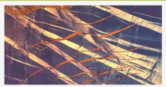
Polarized light microscopy of a Cu-Nb nanolaminate showing poor kink band contrast. From the 2014 IMC Jacquet-Lucas award winning entry.
