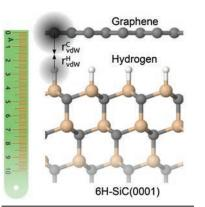
Graphene on a silicon carbide substrate whose surface was treated with hydrogen in order to electrically decouple the graphene. The distance between the two layers, minus the respective van der Waals radii, gives an approximate value for the interaction strength. Courtesy of Sforzini et al., *Physical Review Letters*/The American Physical Society.
