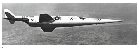
The Douglas X-3 Stiletto was a 1950s experimental jet aircraft manufactured by Douglas Aircraft Co., and the first design to use titanium in major airframe components.
