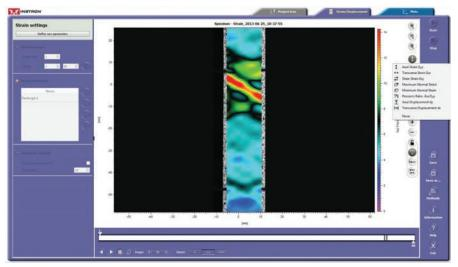
Fig. 3 – Digital image correlation analysis shows localized strain on a metal tensile specimen.
