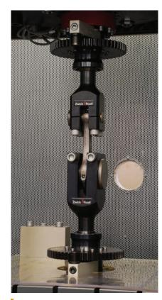
Zwick Vibrophore systems apply the resonance principle to enable fatigue testing of metal specimens. Testing at high frequencies may be done rapidly, enabling greater overall test throughput.
