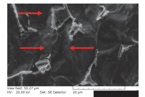
Fig. 5 — SEM fracture surface of bracket showing a mixed fracture mode of shear dimples and transgranular cleavage. Deformation lines (river pattern) on the cleavage surface of crystals are marked by red arrows. Mag: 6000×.
