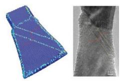
The computer model (left) and experimental image (right) reveal atomic-level deformation twinning in a tungsten nanowire under axial compression. The lattice of the deformation-induced twin band (between yellow lines) is a mirror image of that of the parent crystal. Courtesy of Ting Zhu.
