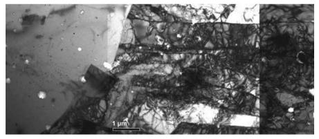
**Fig. 1** — TEM image illustrating the formation of sub-grain structures in AZ31 magnesium alloy when deformed to a strain of ~0.1 followed by annealing at 250°C for 1800 s<sup>[10]</sup>.
