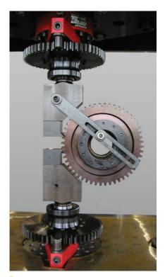
A metal component mounted and gripped for fatigue testing in a Vibrophore system.
