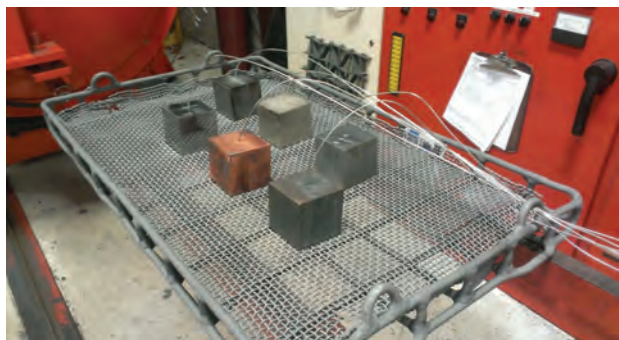
Fig. 2 — Carbon-steel test blocks with inserted thermocouples used to determine the effect of surface condition on times to heat to temperature in a vacuum furnace.
