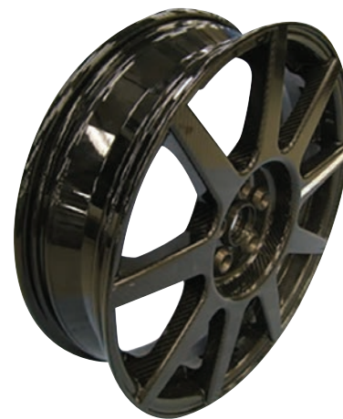
Fig. 6 — MMLV glass fiber composite spring and carbon fiber wheel.
