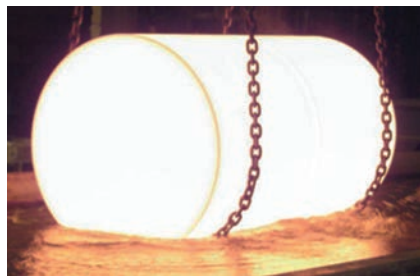
Fig. 1 — Full scale, 1000-mm-diameter alloy 263 rotor forging during solution annealing and quenching. Courtesy of Saarschmiede, Germany.
