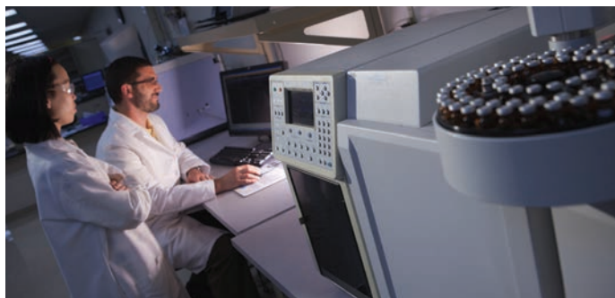
Analyzing samples on the GC-MS in the NSL organic lab.
