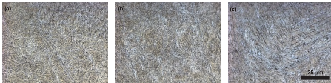
Fig. 3 — QT heat treatment influence on AISI 420 microstructure: (a) Low heat input ( P=200 W, V=1000 mm/s); (b) Moderate heat input ( P=300 W, V=1000 mm/s); and (c) High heat input ( P=300 W, V=800 mm/s).
