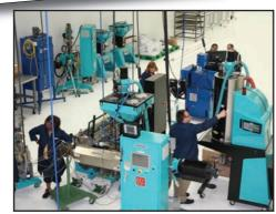
Tri-layer extrusion line for producing high performance tubes and hose.
