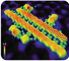
Graphene nanoribbons imaged by scanning tunneling microscopy. Zigzag edges are highlighted by the red structure. Courtesy of Patrick Han.
