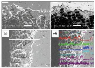
Typical cross-sectional microstructure (a) and corresponding backscattered image of coating Z20Y125 (b); EDS line scanning results of the cross-section of the coating (c, d).
