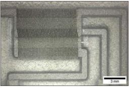
Fig. 3 - Printed heat flux sensors based on differential thermopile design.
