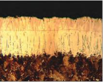
**Fig. 1** — Dual-phase boride layer with FeB (darker "teeth" near surface) and Fe<sub>2</sub>B (lighter teeth). Cracks have formed between the FeB and Fe<sub>2</sub>B layers upon cooling.
