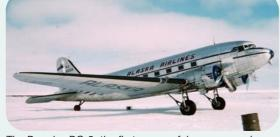
The Douglas DC-3, the first successful passenger plane, was built with 24S alloy, 4% Cu and 1.5% Mg. From 1935 until production ceased in 1945, 18,000 were built for commercial and military use. Public domain image.
