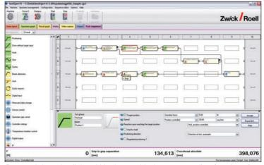
Drag and drop simplicity within the graphical sequence editor function of testXpert II software supports rapid changeover times between tests and helps reduce measurement errors.
