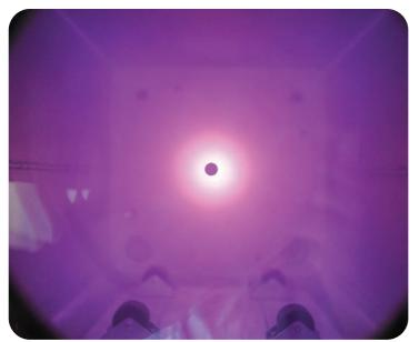
**Fig. 3** — By tailoring the degree of functionalization and achieving optimal dispersion, the low temperature plasma process (>100°C) produces graphene with specific properties and superior performance for customization. Plasma is generated via the central electrode inside the rotating drum.
