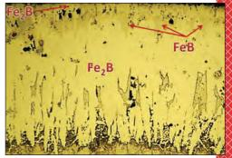
**Fig. 5** — AISI 4140 alloy steel deep case borided to a depth of 0.011 in. followed by a vacuum diffusion treatment. Some FeB near the surface converted back to single-phase  $Fe_2B$  (light colored teeth) while some FeB (darker teeth) is still present at slightly deeper depths. Single-phase  $Fe_2B$  is present below.
