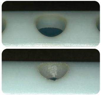
**Fig. 2** — Comparison of 1030-nm fs disk laser (top) to a 355-nm ns laser (bottom) when drilling polypropylene.
