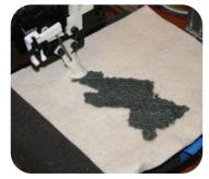
3D printed teddy bear made using a new printer developed by CMU and Disney Research.
