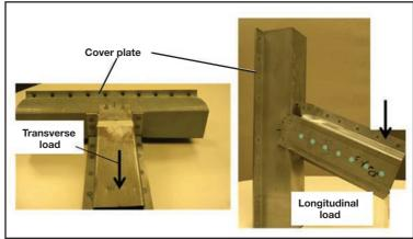
Fig. 9 — Broken T-Section samples.
