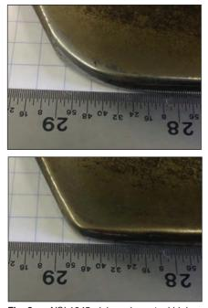
Fig. 8 — AISI 1045 plain carbon steel highwear agricultural machinery parts borided to a depth of 0.005 in. (left) and deep case borided to a depth of 0.014 in. (right). After service on the same machine for the same amount of time, the conventional borided part shows significant material loss due to wear, while the deep case borided part shows virtually no wear.
