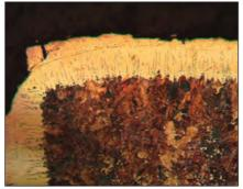
**Fig. 2** — Dual-phase boride layer with cracks between the FeB and Fe<sub>2</sub>B layers. The FeB boride layer at the corner spalled off the surface.
