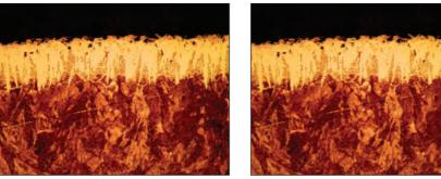
**Fig.** 7 — AlSI 4140 alloy steel ground-engaging tools conventionally borided to a depth of 0.004 in. (left) and deep case borided to a depth of 0.010 in. (right). Boride layers in both are single-phase  $Fe_2B$ .
