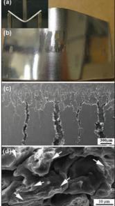
Repaired sample during the threepoint bending test and after 90° bending, respectively (a, b). SEM images at different magnifications revealing the fracture nature that took place during bending (c, d).
