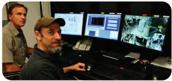
NIST's new calibration service for high-power lasers is controlled from behind a protective barrier. Paul Williams (left) and Joshua Hadler operate the service, which can calibrate lasers with up to 10 kW of power for manufacturers and military customers. Courtesy of Burrus/NIST.
