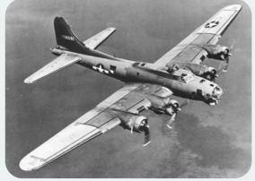
The Boeing B-17 Flying Fortress and nearly all of the 300,000 planes built during WWII used the 24S alloy. The aluminum industry tripled in output to meet wartime demand. Public domain image.
