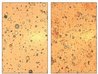
Splats obtained by solution precursor plasma spray from ZrCl-LaNH (a) and ZrCl-LaNEt (27.8 g/L) (b).
