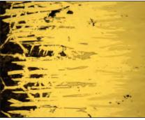
**Fig. 4** — AISI 4140 alloy steel deep case borided to a depth of 0.020 in. using commercially available boriding powder. The boride layer consists of about 50% FeB (dark colored teeth near surface) and 50%  $Fe_2B$  (lighter teeth) below the FeB layer, an undesirable condition prone to spalling.
