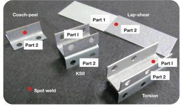
Fig. 3 - Welded versions of small samples.
