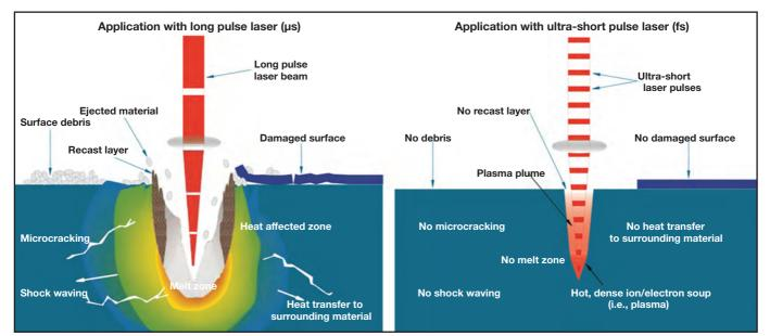
Fig. 1 — Schematic processing comparison of microsecond to femtosecond lasers.
