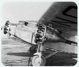
Alcoa's 17S sheet alloy was based on the German alloy, Duralumin, and was used to build the first commercial all-metal passenger airplane in the U.S., the Ford Trimotor. Shown here is the Ford 5-AT-B "City of Columbus" flown by Charles Lindbergh. Public domain image.
