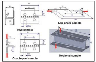
Fig. 1 — Small sample types used to develop spot weld failure parameters.
