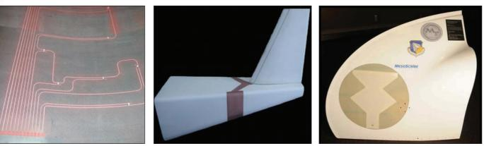
Fig. 5 - Printed copper conductors and antenna patterns. Integrated wiring (left), UHF/VHF/GPS antenna on UAV (middle), structurally integrated VHF antenna onto an aircraft wing to body fairing (right).
