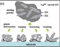
Schematic illustration demonstrates the formation mechanisms of the HA-GN nanocomposite coating.
