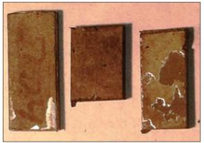
**Fig. 3** — Spalling (small silver-colored relective spots) on three different materials that were borided together: (left) 304 stainless steel, (center) 440C stainless steel, and (right) duplex stainless steel.
