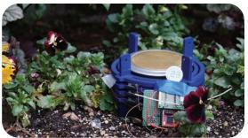
A new thermal power harvester uses naturally changing ambient temperature as its power source.
