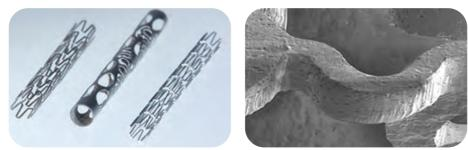
**Fig. 3** — Cut quality for nitinol stent. Nitinol stents (left). Close-up of a 100-µm-thick nitinol stent (right). Edges feature the same finish as the material surface.
