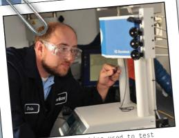
Melt flow index machine used to test polymer viscosities at various temperatures.
