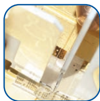
ON THE COVER: Continuous wave-THz spectroscopy system emitter and detector devices for semiconductor materials characterization. Dome-shaped emitters and detectors are mounted on thermally stable, optical stages that maintain THz alignment while measurements are taken at variable temperatures. Courtesy of Lake Shore Cryotronics Inc., lakeshore.com.
