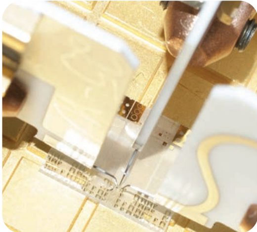
Fig. 3 — Three-terminal DC probing configuration for transistor measurements.
