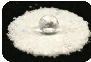
A bead of water sitting on top of water-resistant polymer crystals. Courtesy of Kyoto University.
