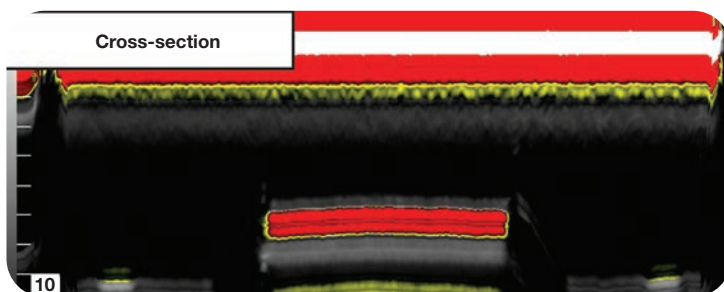
Fig. 4 — Sectioning along line 2 suggests that the delamination is thickest over the center of the die.
