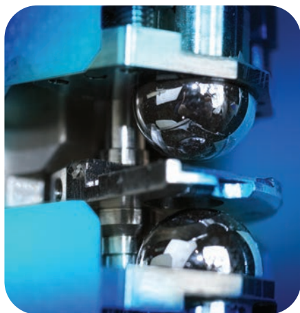
ON THE COVER: Continuous wave-THz spectroscopy system emitter and detector devices for semiconductor materials characterization. Dome-shaped emitters and detectors are mounted on thermally stable, optical stages that maintain THz alignment while measurements are taken at variable temperatures. Courtesy of Lake Shore Cryotronics Inc., lakeshore.com.
