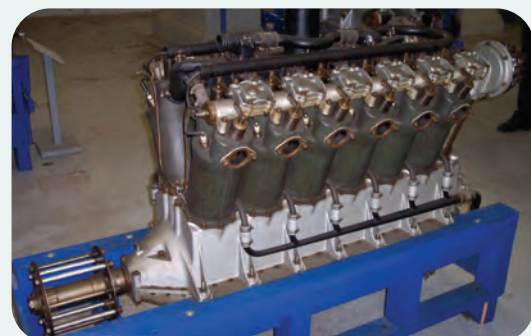
Liberty L-12 aircraft engine. Cast aluminum was used for its light weight. Courtesy of Stahlkocher/Wikimedia Commons.
