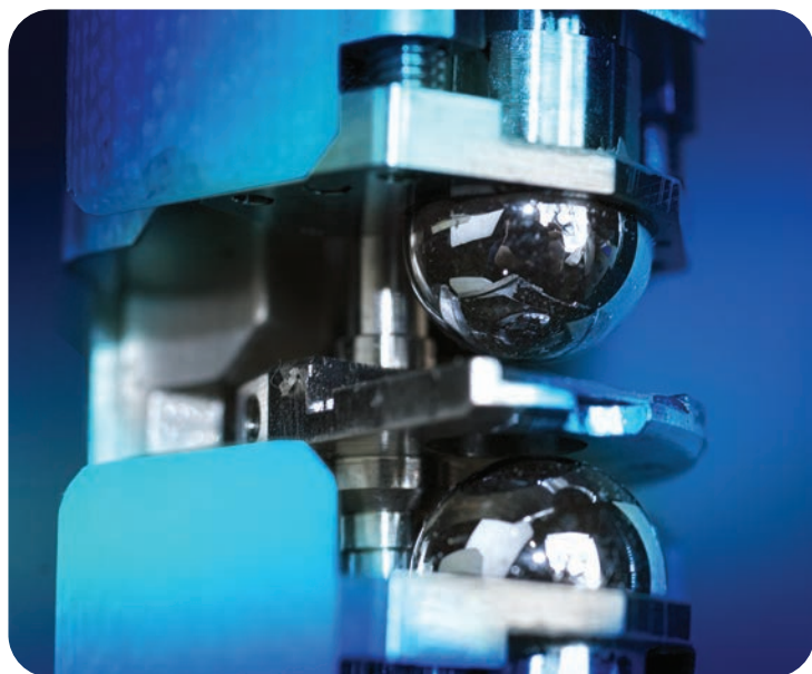
Continuous wave-THz spectroscopy system emitter and detector devices for semiconductor materials characterization.
