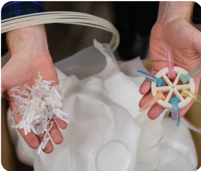
Old milk jugs can be recycled into filament for 3D printing, saving both money and the environment. Courtesy of Sarah Bird/MTU.
