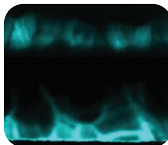
Cross-sectional electron beam-induced current maps show the difference in cadmium telluride solar cells before (pictured above) and after (below) cadmium chloride treatment. The increased brightness after treatment indicates higher current collection at grain boundaries. Courtesy of ORNL.
