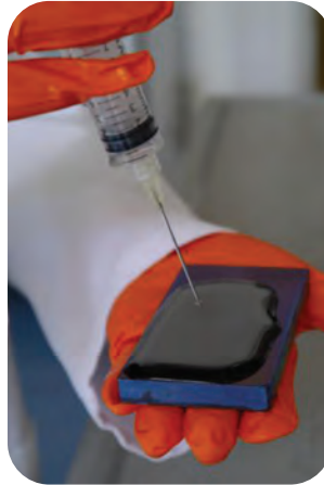
A gel-coated titanium surface binds proteins that promote bone formation. Courtesy of Ida Berts.
