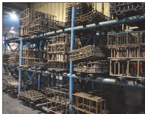
Furnace fixtures at various levels of degradation.
