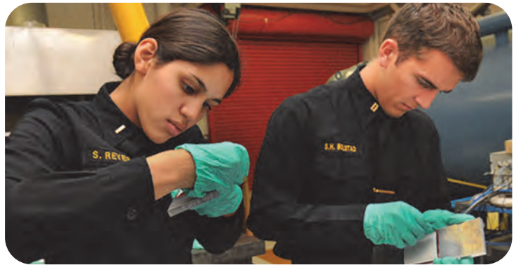
Fig. 3 — MIDN Sabrina Reyes and Scott Bolstad conduct corrosion fatigue research on composite repairs of aluminum alloys for aerospace and naval ship applications. Courtesy of CorrDefense DoD News.
