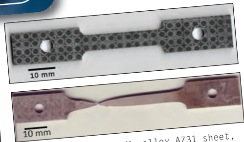
A sample of wrought Mg alloy AZ31 sheet, before (top) and after high-temperature tensile testing, shows the effect of heat as well as strain. Results are being used to help build open data repositories where researchers can easily distribute and share data.
