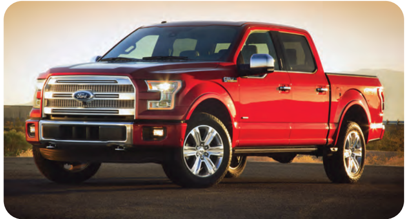
Fig. 2 — The 2015 Ford F150 boasts a body comprised of aluminum alloys, reducing truck weight by 700 lb.
