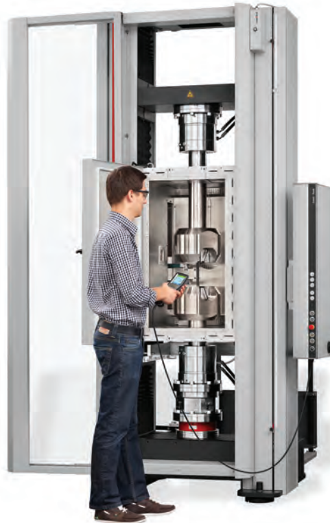
Fig. 5 — Zwick's Allround-Line system supports testing of aluminum, magnesium, specialized alloys, and composites. Dual testing areas improve efficiency by reducing changeover time.
