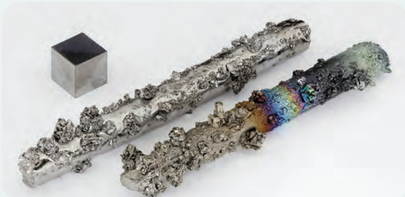
99.98% pure tungsten rods with evaporated crystals, partially oxidized with colorful tarnish; high-purity tungsten cube for comparison. Courtesy of Alchemy-hp/Wikimedia Commons.
