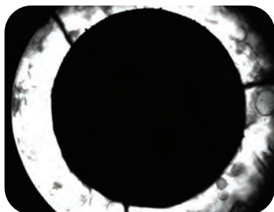
Fig. 2 — Super-compressed CO 2 at pressure and temperature surrounding the elastomer during decompression.
