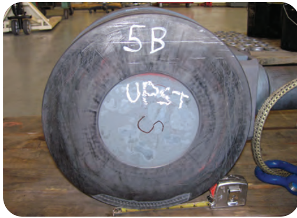
Fig. 1 — Delamination of hardfacing material from a ferritic valve disc operating in a cycling, gas-fired power plant at 1050°F after roughly 35,000 hours.
