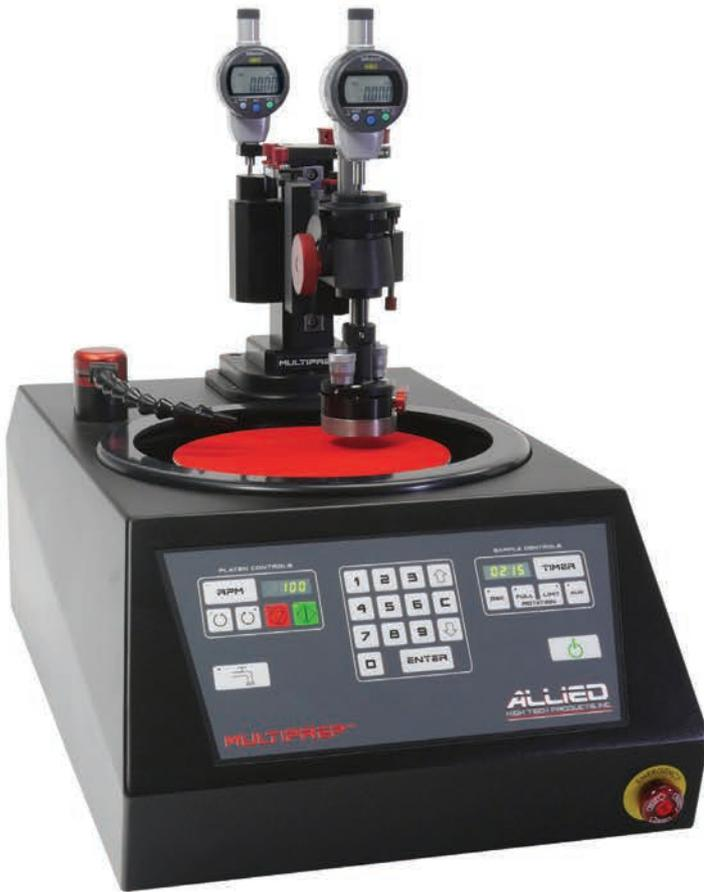
The **MultiPrep™ System** enables precise semiautomatic sample preparation of a wide range of materials for microscopic (optical, SEM, FIB, TEM, AFM, etc.) evaluation.
