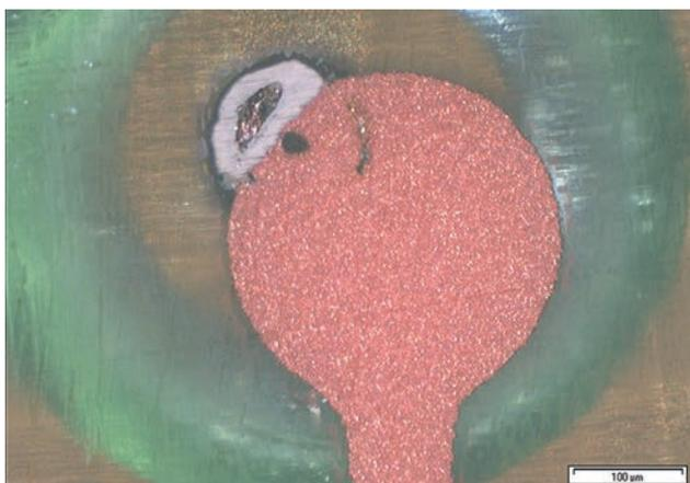
**Fig. 8** Magnified view of Fig. 7 showing detail of the misalignment
