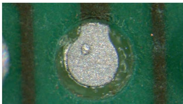
**Fig. 6** The footprint of the dropped-out ball shows that there was a problem with a clogged stencil mask while printing the solder paste. Just one small solder bead was transferred to the pad.
