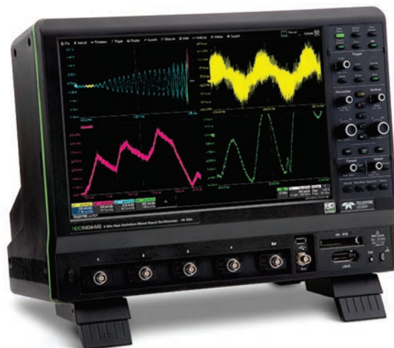
Teledyne LeCroy's HDO9000 high-definition oscilloscope
