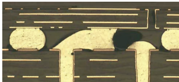
Fig. 4 Cross section of the solder faults from Fig. 3. Short circuits caused by flowing solder as a result of missing solder resist
