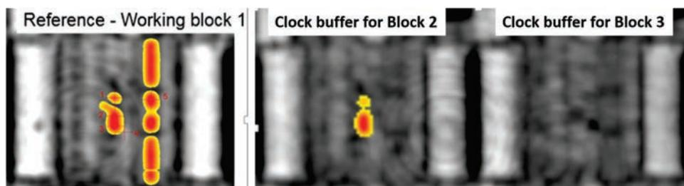
**Fig. 7** LVI images at the clock buffers (D clock) for block 1 (reference), block 2, and block 3
