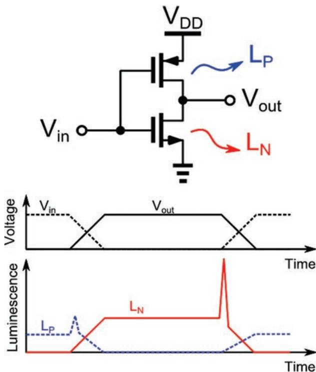
**Fig. 2** Example of luminescence signal (L) from a simple inverter gate. With TRE, it is possible to retrieve both the logic state of the gate (the gate is leaking when it is off) and when it turns on (in correspondence of the switching emission peak).
