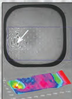
NIR image top shows the thinnest area on a thinned- deliberately tilted die. Lower image shows a C-SPM scan made on ASAP-1 IPS of the same area showing a consistent point of minimum RST.
