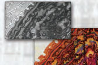
NIR and VISIBL Images show the same position as the Plot screen for silicon breach
