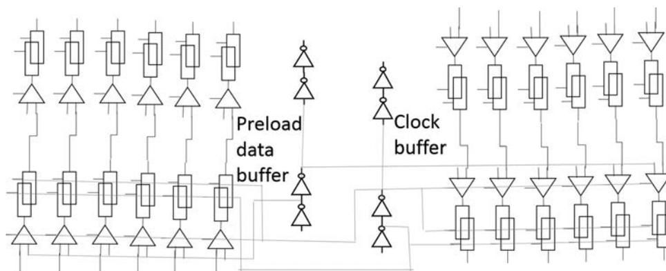
**Fig. 3** Diagram of scan chains in a pack showing the latches at the same position for six scan chains in a pack that share the same preload data buffer and clock buffer
