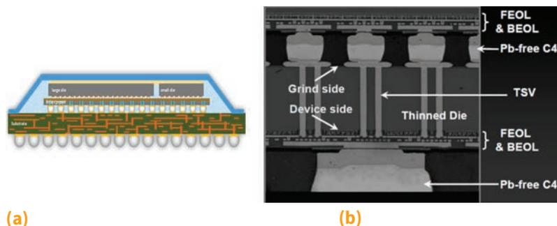
**Fig. 1** (a) Example of 2.5-D integrated system-in-package based on interposer technology.<sup>[2]</sup> (b) High-magnification image of interconnection realization between full die (top), thinned die (middle), and laminate (bottom) using TSV, micropillar, and thinned-die packaging.<sup>[3]</sup>
