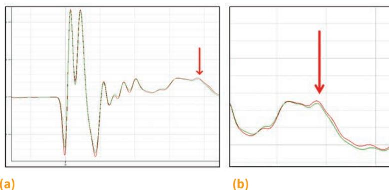
**Fig. 9** (a) EOTPR measurement overview and (b) high magnification of reference (green) and failing (red) device signatures. A slight difference is noticeable after the signal passes the ball-grid array contact and laminate.
