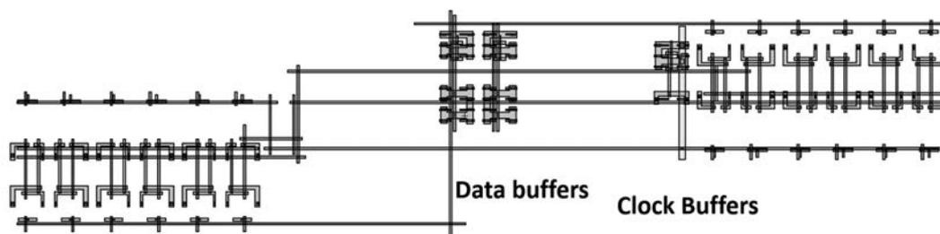
**Fig. 10** Layout tracing that shows these latches at the same position in different scan chains in a pack are sharing the same clock buffer and data buffer
