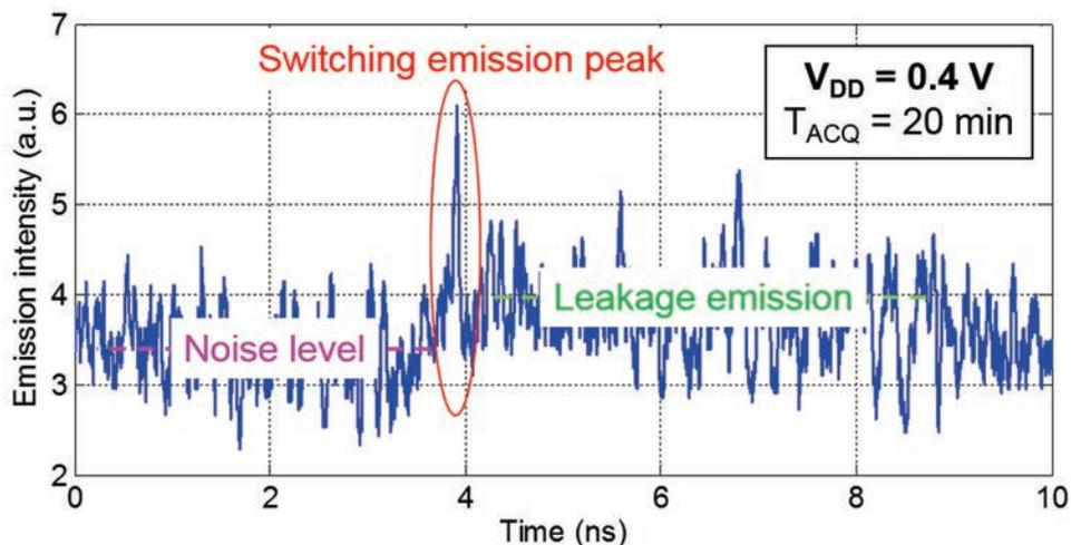
**Fig. 6** Ultra-low-voltage TRE measurement acquired from an inverter chain fabricated in IBM SOI 32 nm technology.<sup>[10]</sup> The leakage emission can be distinguished from the noise level, and the switching emission peak can be easily identified.
