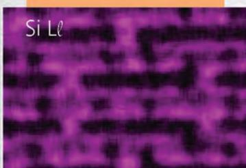
With just two 6 minute maps it is possible to fully characterize a bulk semiconductor device. At 3 kV all elements in the specimen can be resolved to sub 20 nm resolution. At 1 kV light elements can be mapped with high surface sensitivity and 10 nm lateral resolution.
