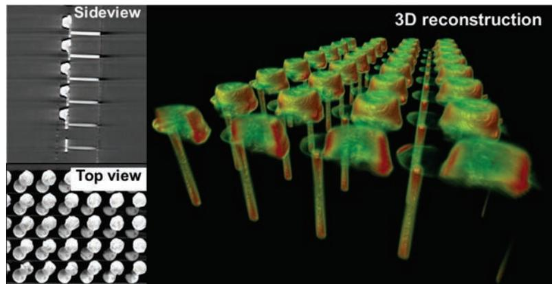
**Fig. 10** 3-D x-ray results showing a misalignment between microbumps and TSV features
