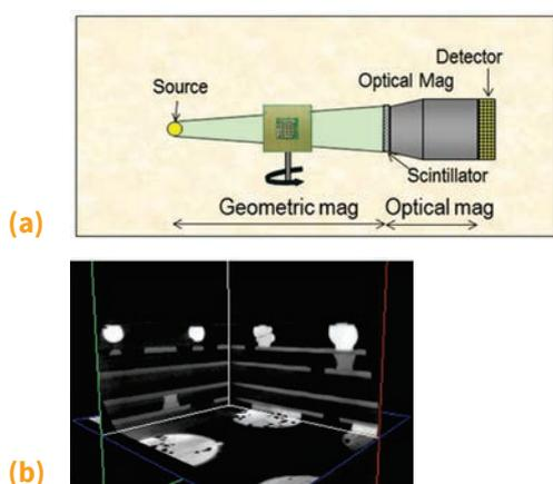
**Fig. 2** (a) Operational principle of 3-D x-ray. Using sample rotation, several 2-D x-ray images are taken and processed. (b) As a result, a 3-D model is created that allows selective “virtual cross sectioning” of any desired x-y-z-layer.
