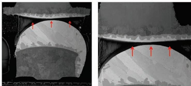
**Fig. 8** Plasma FIB cut through a failing bump confirms the 3-D x-ray results and root-cause theory of an unlanded microbump.
