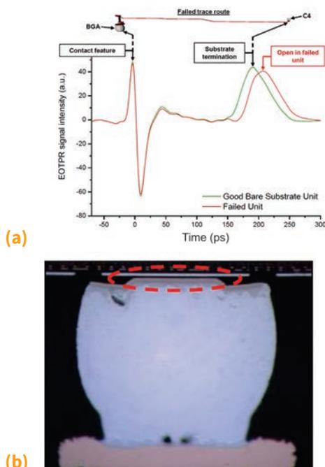
**Fig. 3** (a) Introducing a high-frequency signal into the sample and measuring the time of flight of the reflected response allows a simple reference-versus-failing device comparison. (b) Cross sectioning and root-cause imaging of an open C4 bump after successful EOTPR measurement
