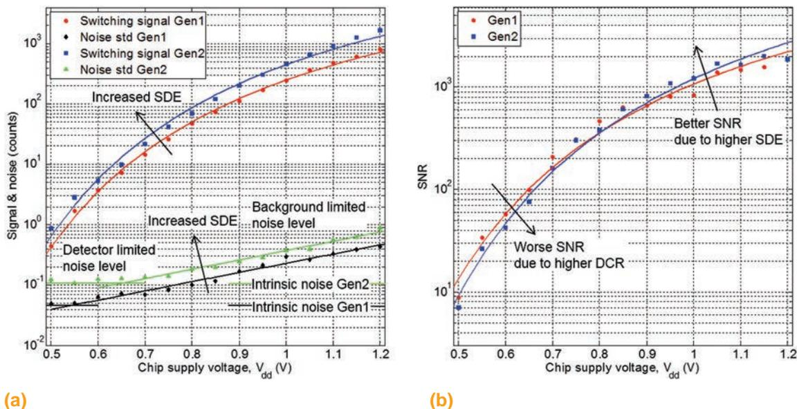
**Fig. 5** (a) Switching emission signal and noise as a function of chip supply voltage for two different generations of SSPD.<sup>[10]</sup> The noise at low voltage is limited by the detector noise, while at high voltage it is limited by the background (i.e., light coming from neighboring devices). (b) Signal-to-noise ratio (SNR) as a function of supply voltage for the two detectors.<sup>[10]</sup> SDE, system detection efficiency; DCR, dark-count rate
