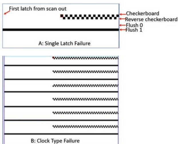
**Fig. 5** Examples of (a) single-latch and (b) clock-type failures
