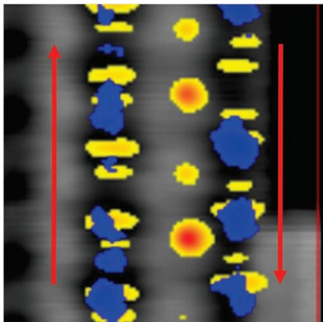
**Fig. 2** Example of LVI image for a scan chain: blue for data signal, yellow for clock signal, and red arrows for data propagation direction
