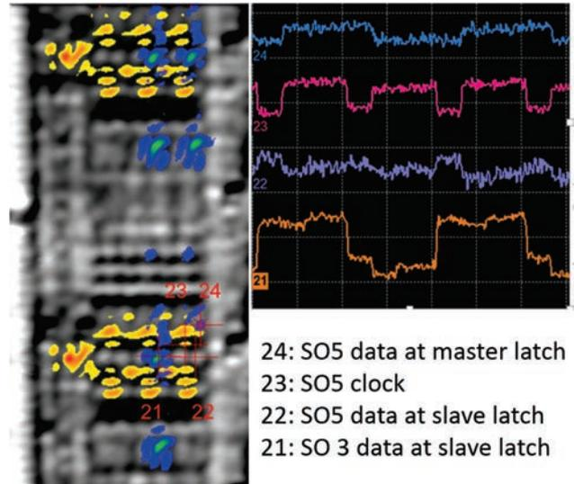
**Fig. 16** LVP waveforms from the master latch of the latch callout, the slave latch from the latch callout, and the adjacent reference latch, indicating data missing at the slave latch for the latch callout
