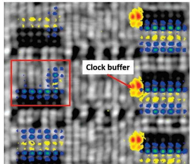
**Fig. 12** Magnified LVI image of Fig. 11 shows a strong clock signal at the clock buffer and some data signals for the latches close to the clock buffer, and no data signals for the latches far from the clock buffer.
