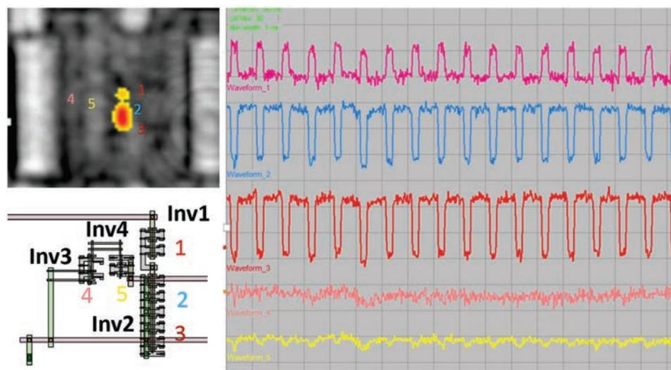
**Fig. 8** LVP waveforms collected from five points marked in the layout clip of the cascaded inverters
