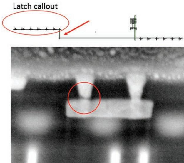
**Fig. 14** FIB cross section showing hollow V2 in the clock signal line from the clock buffer to the latch callout
