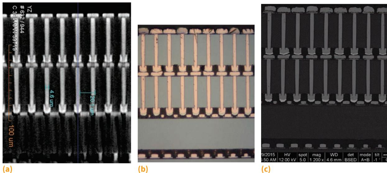
**Fig. 1** Comparison of (a) virtual cross-sectional image obtained by XRM and (b, c) optical and SEM images taken after physical cross sectioning for 20- $\mu\text{m}$ -pitch TSVs (5  $\mu\text{m}$  diameter) and bump joints. Images by Carl Zeiss X-Ray Microscopy, Inc.; sample from imec. Figure from Ref 3, with permission from SMTA and Chip-Scale Review
