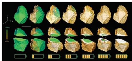
**The chemical phase within the battery evolves as the charging time increases. The cut-away views reveal a change from anisotropic to isotropic phase-boundary motion.**
