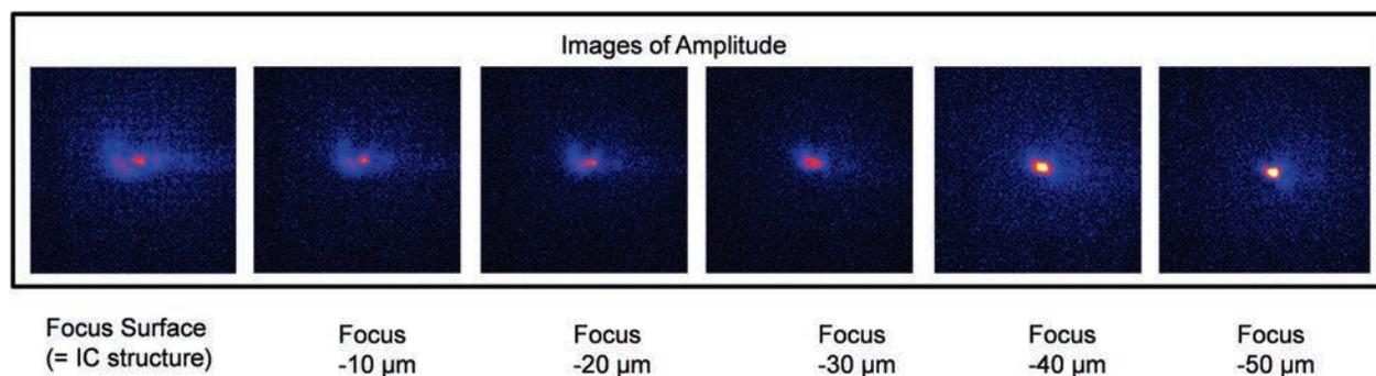
**Fig. 3** Backside LIT images with SIL taken of a breakdown spot of a 5- $\mu\text{m}$ -diameter, 50- $\mu\text{m}$ -deep copper TSV at different focus positions. The images clearly indicate that the breakdown is located close to the bottom of the TSV (focus  $-50\ \mu\text{m}$ ). Measurements by C. Grosse and F. Altmann, FhG CAM, Halle, Germany; sample from imec
