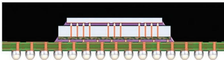
**Fig. 5** Schematic drawing of wide I/O on logic dice with TSV
