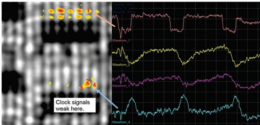
**Fig. 13** LVP waveforms of the input clock circuitry inside the latch callout show a weak clock signal compared to the one from the reference latch.
