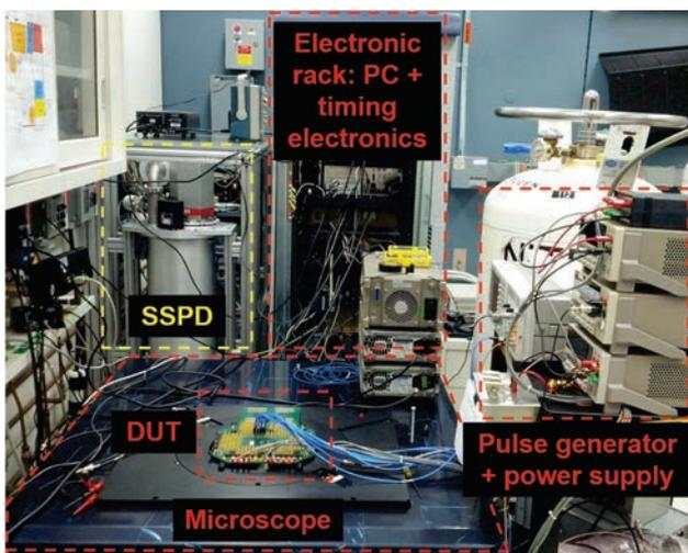
**Fig. 4** Experimental setup used to acquire TRE waveforms
