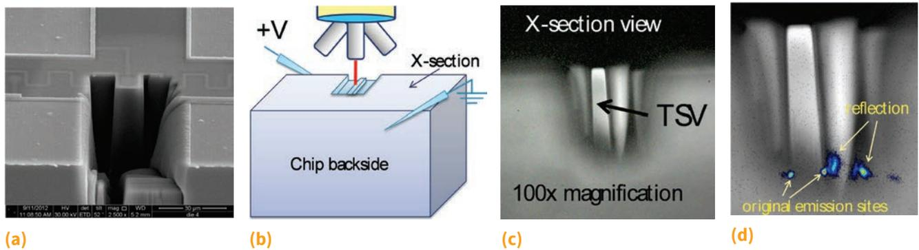
**Fig. 5** In situ localization of the breakdown site of the liner of a 5- $\mu\text{m}$ -diameter, 50- $\mu\text{m}$ -deep copper TSV. (a) Sample prepared by cleaving and FIB, leaving silicon near the TSV. (b) Schematic showing the sample in the PEM setup and the probing from the sides. (c) Cross-sectional microscopy image taken with the PEM setup. (d) Overlay image showing emission detected near the bottom of the TSV. Some light is reflecting from the side walls of the FIB-cut hole.
