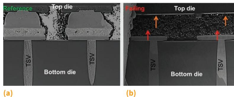
**Fig. 11** Plasma FIB cut through x-ray-investigated area for (a) reference and (b) failing devices. High-magnification scanning electron microscopy imaging confirmed missing die-die interconnection as the root cause.
