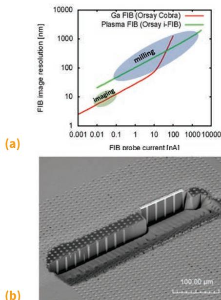
**Fig. 4** (a) Comparison of resolution versus current for Ga-FIB and plasma FIB. (b) Demonstration of TSV cross sectioning
