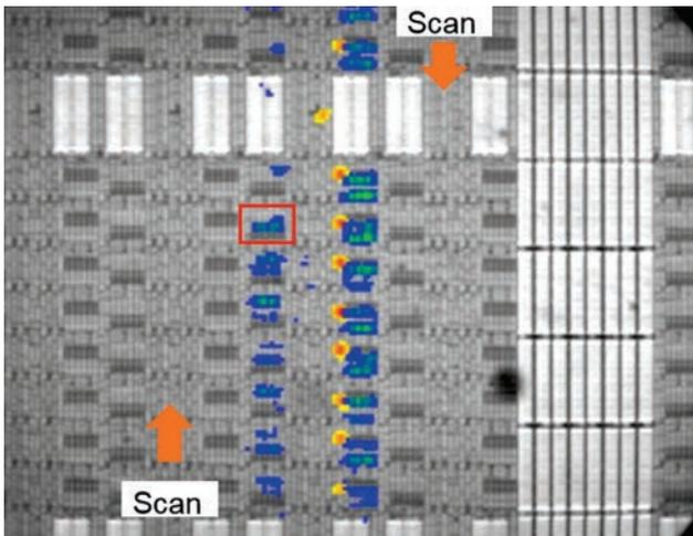
**Fig. 11** LVI image of the six scan chains with clock-type failure in a pack. The red square indicates the latch callout position.
