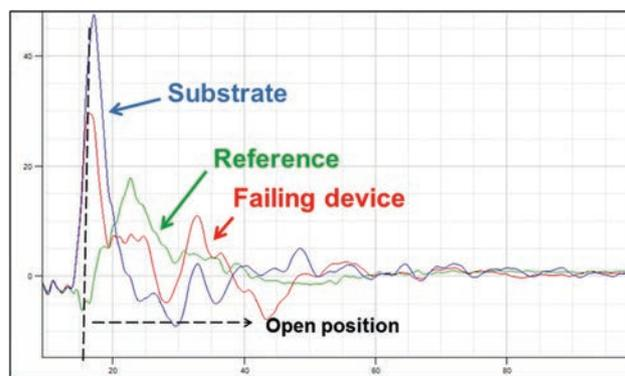
**Fig. 6** EOTPR results on failing device, reference, and bare substrate indicate a defect located in the die-substrate interface
