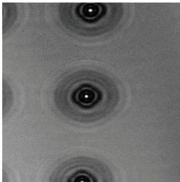
**Fig. 2** Rayleigh fringes observed near 5- $\mu\text{m}$ -diameter TSVs using a GHz-SAM system. Experiments done at FhG CAM Halle, Germany; sample from imec; PVA TePla system
