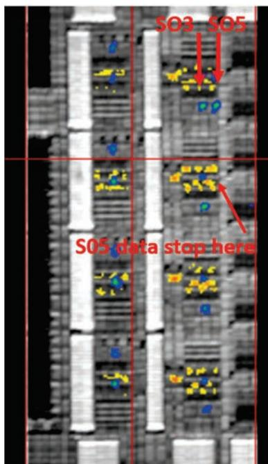
**Fig. 15** LVI image of data signal and clock signal for a reference scan chain, SO3, and the failing scan chain, SO5, indicating a broken point at the latch callout for the failing scan chain, SO5
