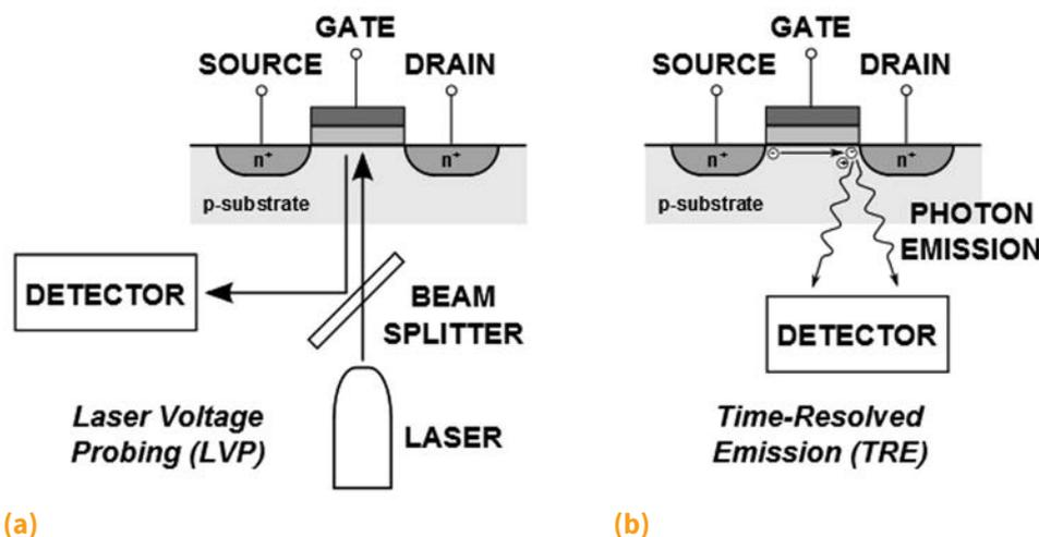
**Fig. 1** Comparison of the two main optical techniques used to detect timing-related faults within an IC. (a) In LVP, a laser is shined toward the device, and the reflected light is modulated by the carriers and detected by a detector. (b) In TRE, NIR photons are spontaneously emitted by the IC and collected by the detector.
