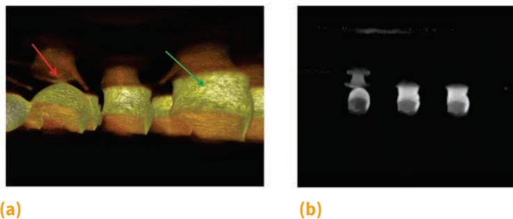
**Fig. 7** (a) 3-D x-ray and (b) virtual cross section identify the root cause of the electrical open as a nonwet microbump.
