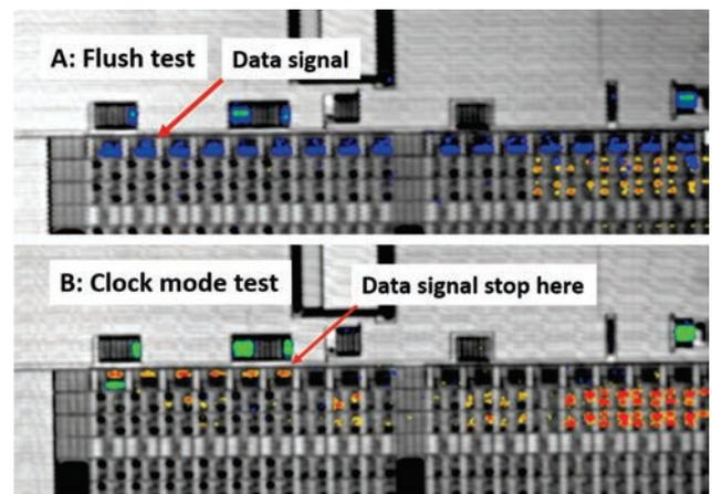
**Fig. 6** LVI image for the skip test scan chain. (a) Flush test. (b) Clock mode test
