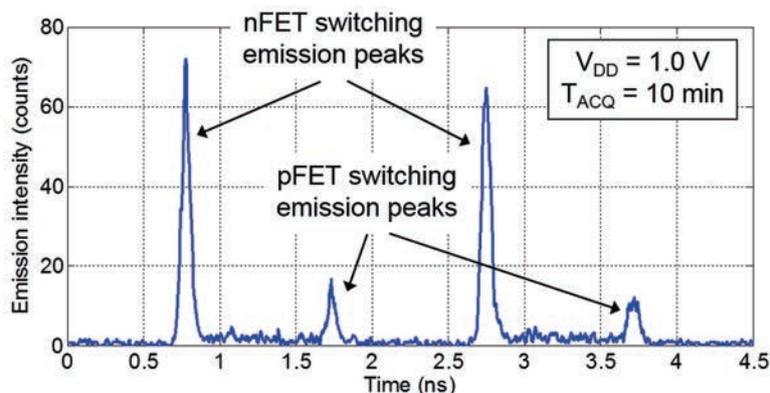
**Fig. 7** TRE waveform acquired from an inverter of a 100-stage IBM 14 nm FinFET SOI ring oscillator. The light is collected from a single inverter. The switching emission peaks from both the *n*FET and *p*FET are visible.
