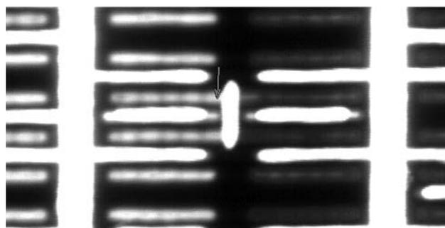
**Fig. 9** SEM image showing a short between the source/drain contact and the gate contact at inverter 3
