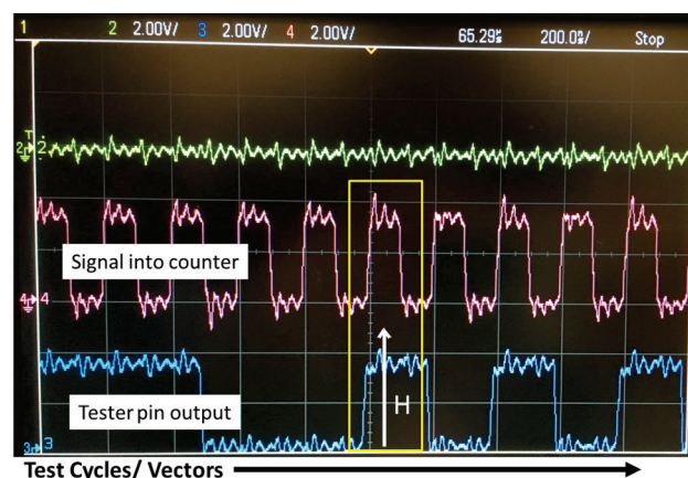
Fig. 3 Synchronizing signal and output pin waveforms viewed from an oscilloscope
